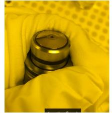
Using the pipette, deposit one droplet of IPA on the lens. The liquid will flow and be absorbed by the tissue. Blow dry the lens with N2 gun. Repeat two-three times until the lens seems clean. PGMEA can be used if IPA is not effective enough.
