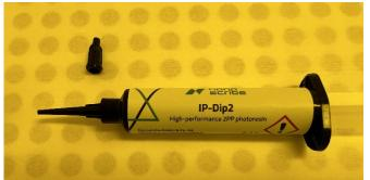
Dispense one drop at the sample center by gently pushing the cartridge piston. Spread out if necessary. After use, the tips should be cleaned after use by immerging in PGMEA for ~20 minutes and rinsing with IPA. EPFL Center of MicroNanoTechnology EPFI
