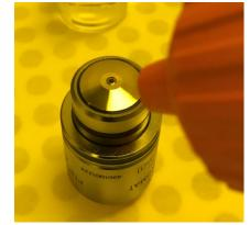
STEP 3: Wrap one tissue around your index, hold the lens firmly and tilt it slightly as shown below.
