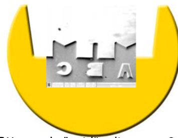
TEM sample "grid", diameter 3mm
