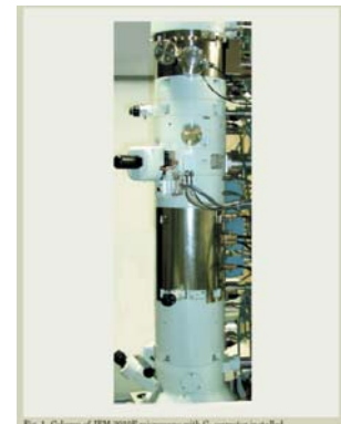
Fig. 1. Column of ZEM-1010F microscope with C_s corrector installed.
