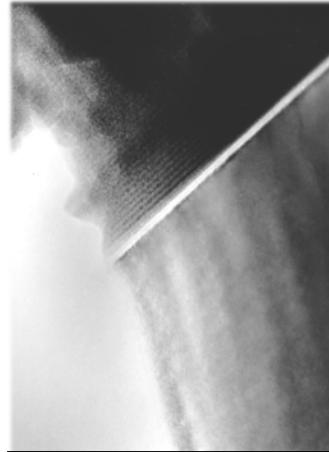
Cr-Ti 50-50/Si substrate Supposed to be columnar grown EELS confirmed Cr-Ti layers
