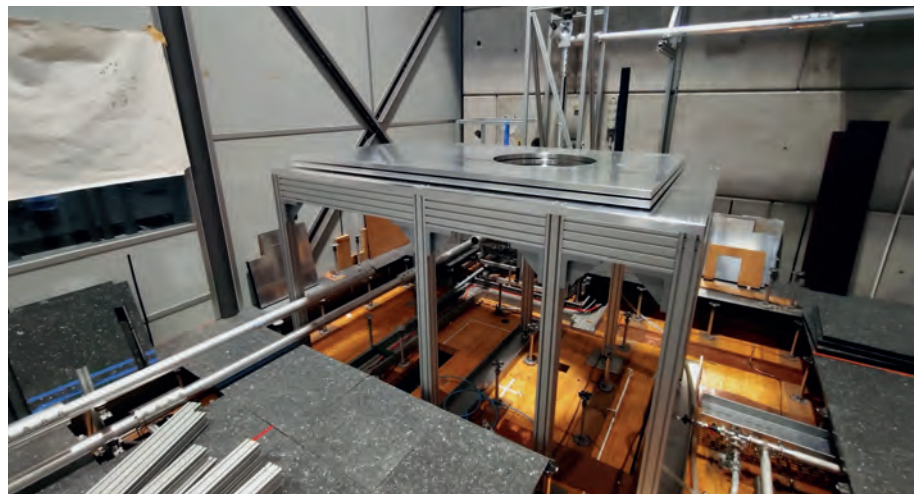
3 Tower of the future G12 bi-frequency gyrotron during its assembly phase.
