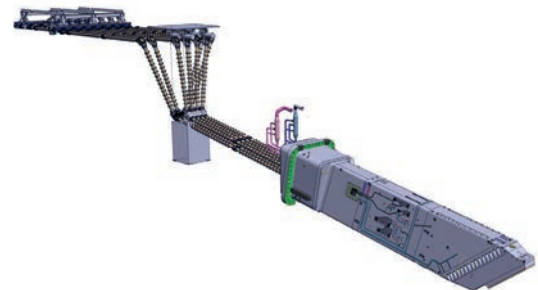
4 The ITER Upper Launcher with ex-vessel waveguide transmission lines (TLs) attached. The last mirrors (M4s) direct 8 beams (4 each) into the plasma to drive current to stabilize the neo-classical tearing modes and avoid potentially damaging plasma disruptions.
