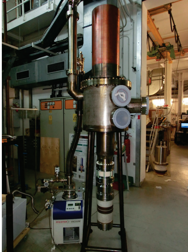
Fig. 2.5.1 Picture of the short pulse gyrotron before its installation in the superconducting magnet.
