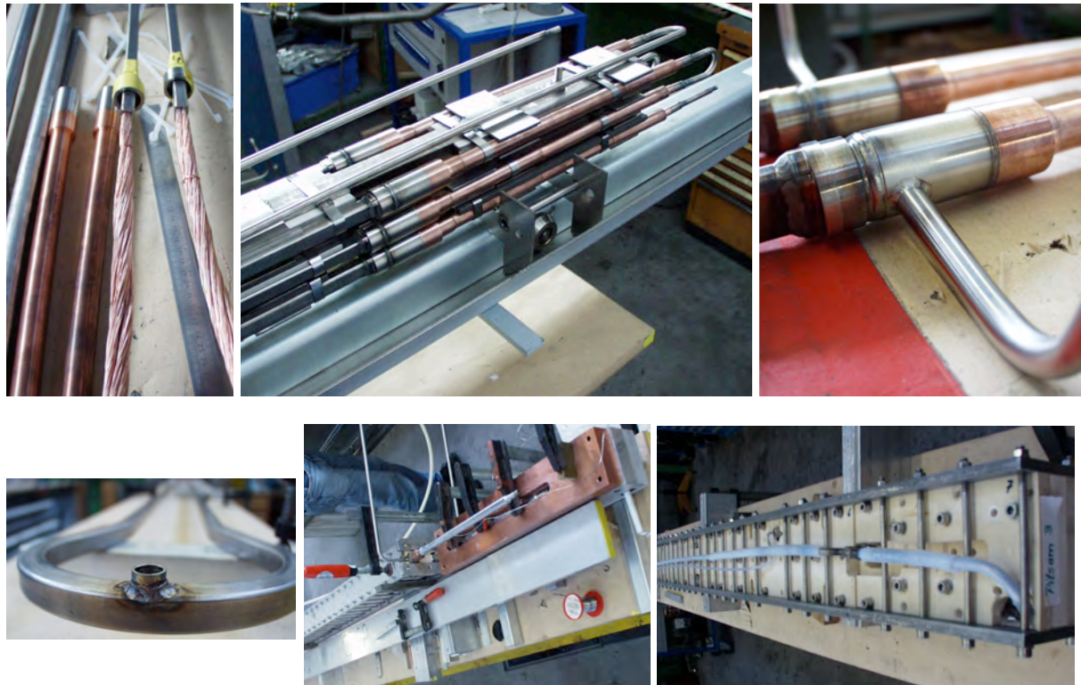
Fig. 2.5.12 Preparation of the PITSAM samples. From top to bottom: the dismantled conductor ends after removal of Cr coating (left the steel/copper sleeves), PITSAM2, 3 and 4 prepared for heat treatment (termination side), detail of the helium outlet next to the termination, penetration for the helium inlet at the U-bend, soldering of the termination into the thick copper plate, sample in the clamp with piping and sensors.
