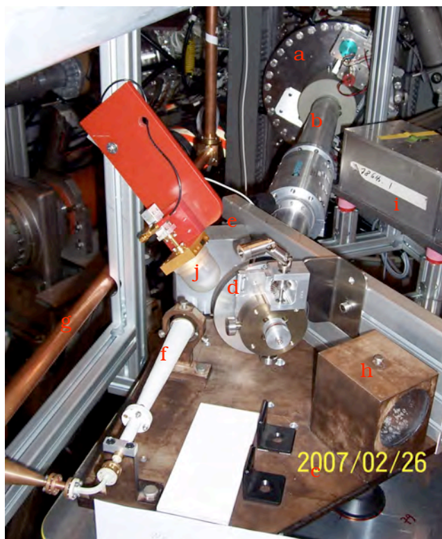
Fig. 3.2.10 Oblique ECE receiver: (a) motorised launcher, (b) HE11 waveguide, (c) adapter baseplate, (d) grating mirror, (e) focusing mirror, (f) scalar horn, (g) 25mm waveguide to LFS radiometer, (h) HE11 waveguide connection for adapter orientation when used for reflectometry, (i) reflectometer source/detector and (j) omni-directional detector for security against gyrotron radiation.
