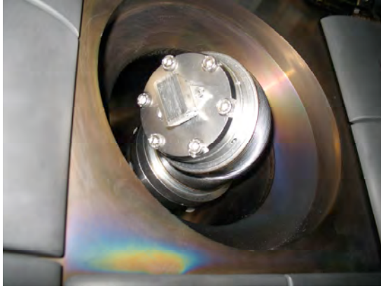
Fig. 3.2.5 View of the X-Ray diagnostic head from inside the vessel. The system is rotated to a typical near-tangential viewing direction. The outer set of Soller plates is visible.
