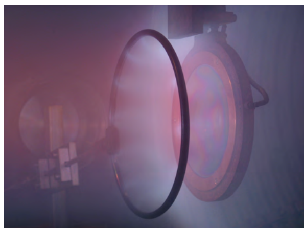
Fig. 2.6.5 Methane injection into a plasma torch jet
