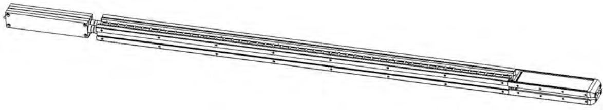
Fig. 2.5.8 A SULTAN sample of ITER TF conductor after final assembly.
