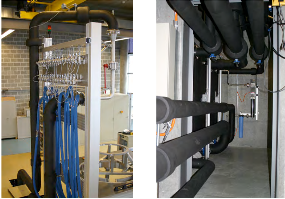
Fig. 3.6.6 Left: Collector circuit with collector simulation valve and hoses of the auxiliary circuits ready to be connected. Right: Main piping to and from the tanks, disinfection unit.
