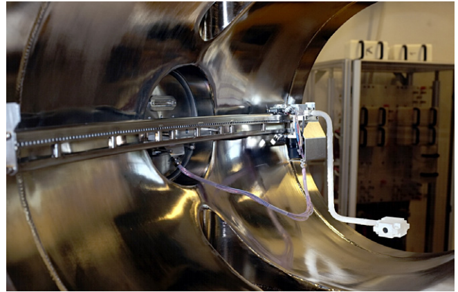
Figure 1. Photograph of the fast ion source mounted on the toroidally movable system in one of the TORPEX sectors. The source is positioned in the lower part of the device to maximize the distance traveled by the ions before they reach the upper wall because of their vertical drift.
