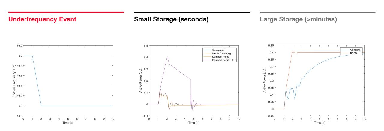
**Converter Based Storage and Generation can Emulate Inertial Response of Synchronous Machines**
