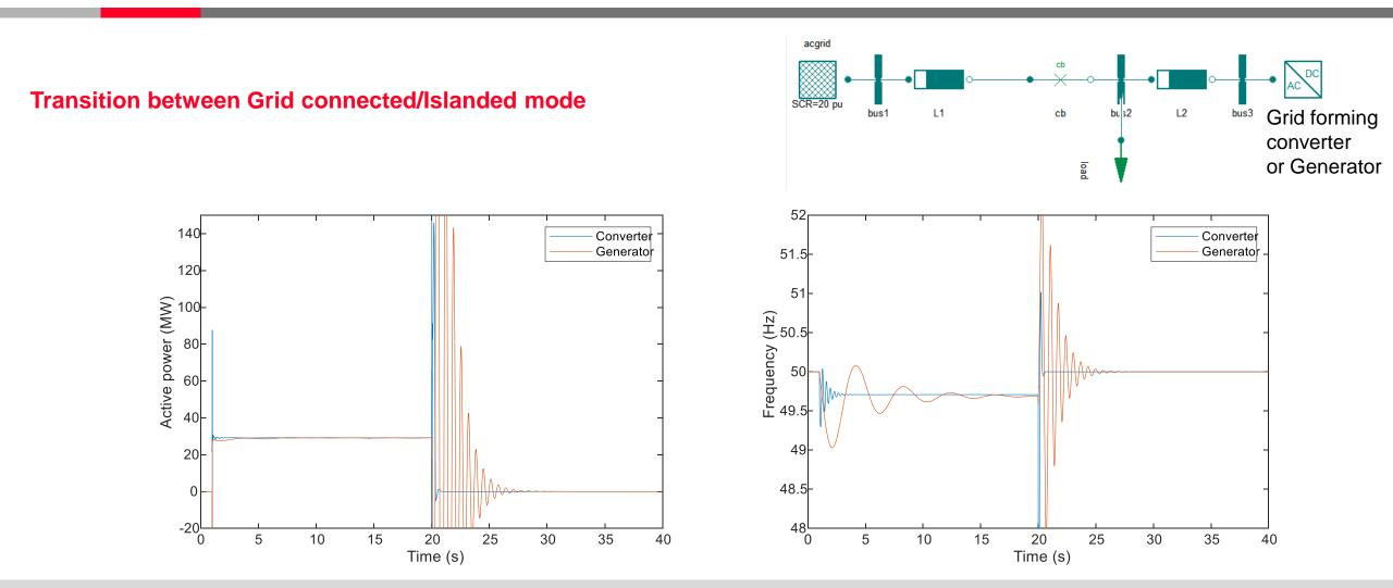
Converter Based Storage and Generation Can Respond Smoother and Quicker in Islanding and Resynchronization
