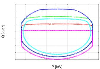
PQ capability curves as function of the real-time BESS status & grid status
