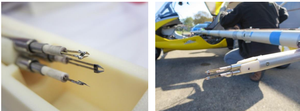
Figure 35: T-NSTAPs mounted on the side of the ULM fuselage.
