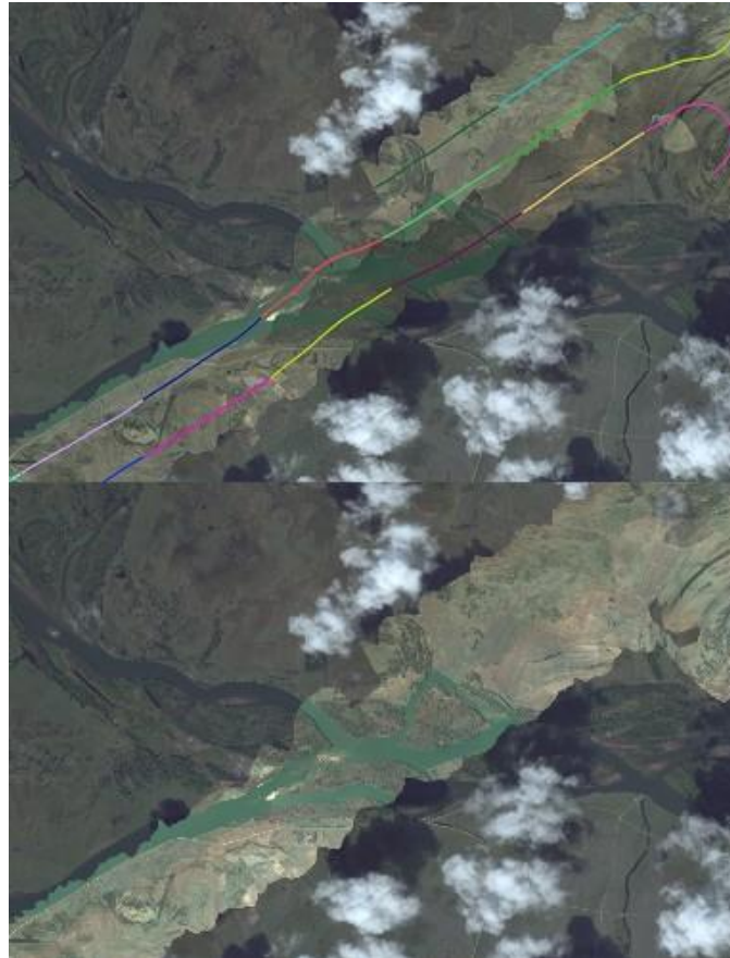
Figure 11: example of light intensity correction: top image represents a flight visualized in HypOS before correction, and bottom image illustrates the same after correction.
