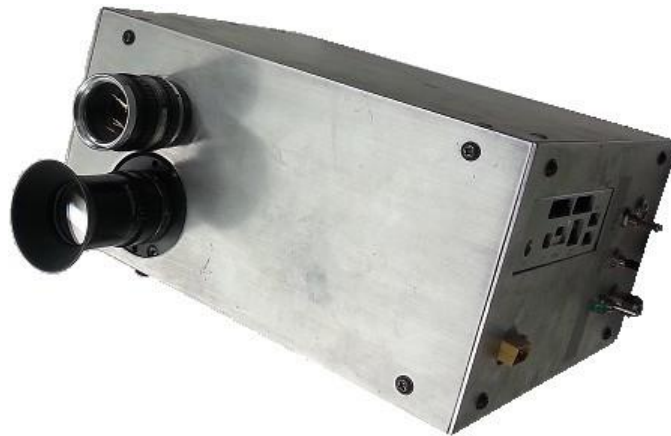
Figure 1: our system contains a hyperspectral camera, an RGB camera, and navigation sensors to georeference the images.
