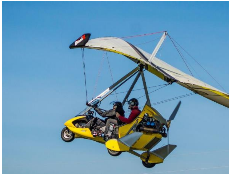
Figure 3: Air Creation Tanarg 912S ultralight aircraft with the remote sensing platform installed
