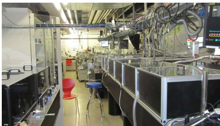
Figure 2. Harmonium: The High Harmonic Generation (HHG) source of pulsed vacuum ultraviolet radiation used for time-resolved photoelectron (gas, liquid solids) spectroscopies at LACUS.
