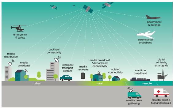
Interconnected satellite 5G network (adapted from Giambene et al., 2018)
