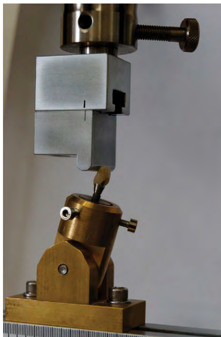
Typical testing machines that subject dental implants to the same chewing conditions experienced by natural teeth.
