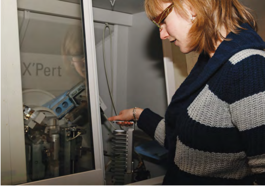
A. Bazzoni places a cement sample into the X-ray diffractometer to assess its crystal structure.
