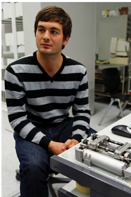
D. Muff performs tensile testing with a stage that can also be used in-situ with various microscopes.
