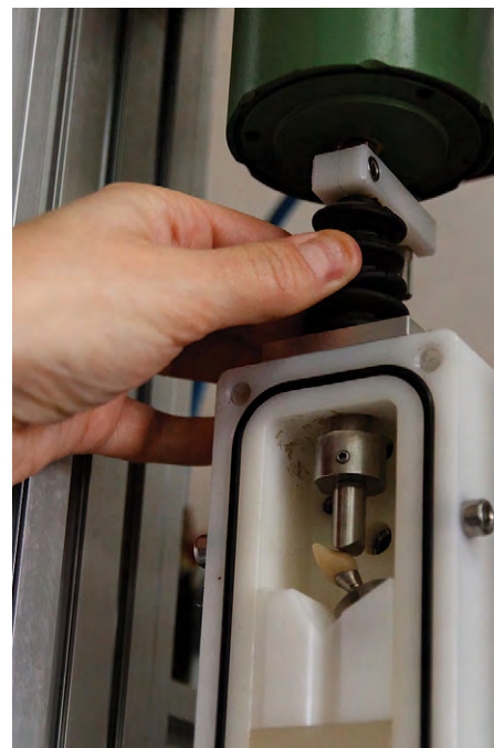
Typical testing machines that subject dental implants to the same chewing conditions experienced by natural teeth.
