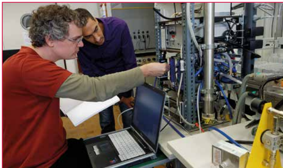
A. Hess and M. Tarik have to precisely tune the gas flows on the modified SMPS at startup.
