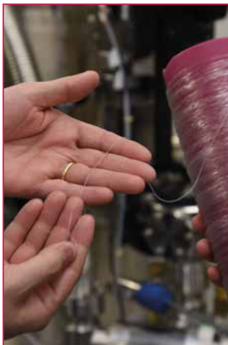
Illustration of polymeric optical fibre flexibility.
