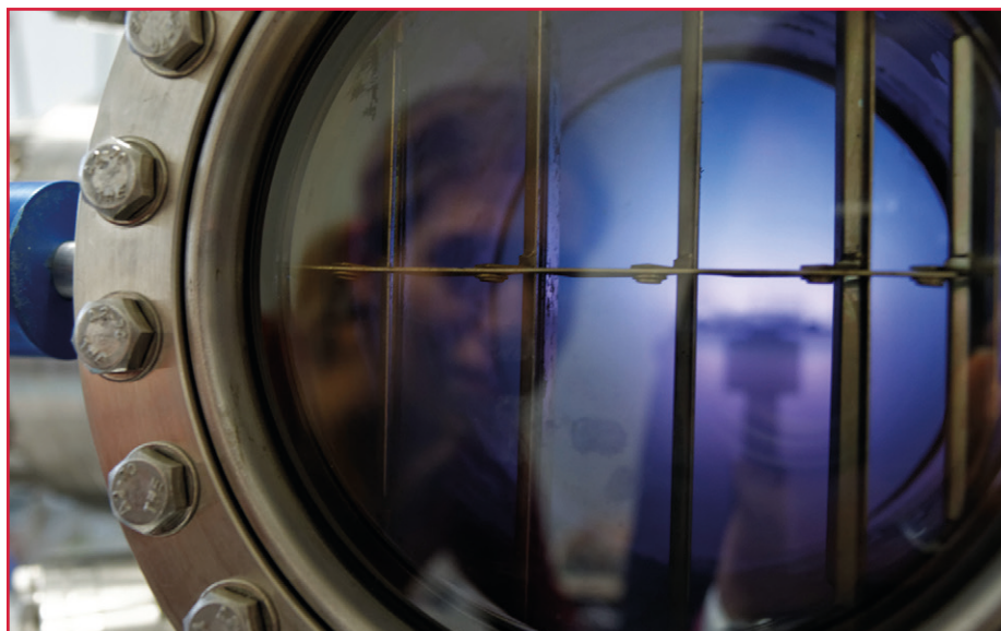
CCMX project researcher monitors the progress of an Argon plasma cleaning of a sample, Empa.
