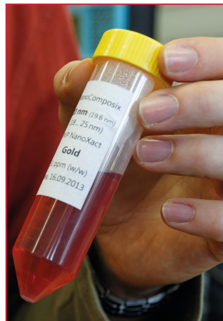
Suspended gold nanoparticles used to generate model aerosols for instrument validation.
