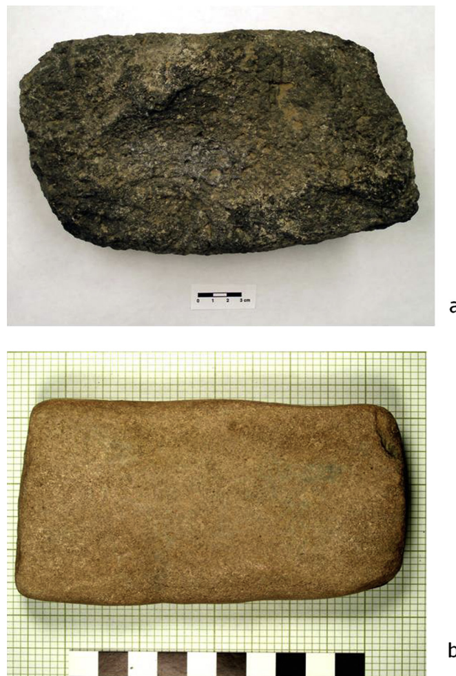
Fig. 1. Macrotopography: (a) naturally rough and angular surface on a vesicular rock; (b) flat surface on a granular rock that is asperite enough to abrade a contact surface.
