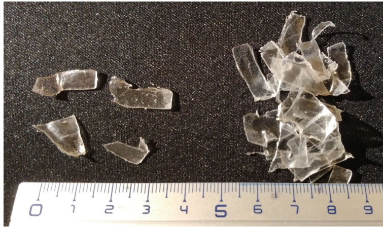
Figure 13: Shredding product of PET bottles
