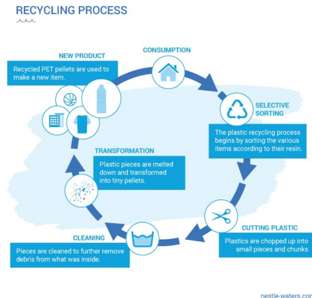
Figure 1: Steps of PET recycling
