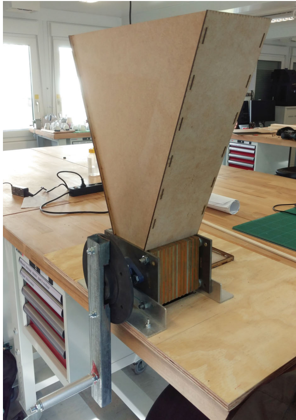
Figure 12: Build of the shredder completed with Hoper and handle
