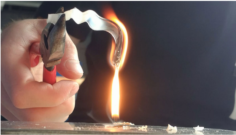
Figure 7: Flame test with HDPE
