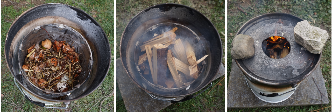
Figure 3: The working principle of the stove: fresh biomass is filled in the bottom of the stove, wood is added on top of it, lit on, and once it burns well, the lid is put on.
