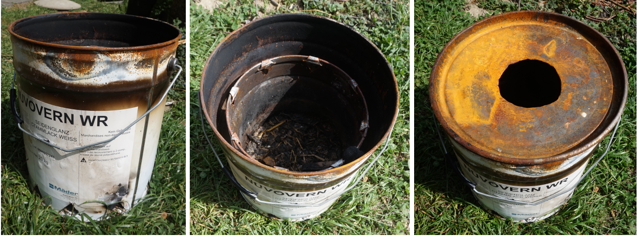
Figure 2: The biochar stove produced: two layers of cans with an aeration system from the bottom and holes for pyrolysis gases to escape on the top of the inner can. Finally, the lid with a hole in the center aims to maximize the heat in the stove while ensuring a sufficient flow of oxygen for the fire.
