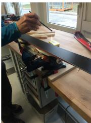
Then, remove the melted holmenkol folit which exceeds the sole with a rigid metal plate, scrape and smooth the sole (this equalizes the ski sole). Always scrape from top to the end of the ski.
