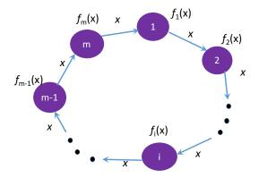
Solving  $\min_{x \in \mathbb{R}^n} \frac{1}{m} \sum_{i=1}^m f_i(x)$  with a cyclic incremental method. Each iteration consists of an update of x along a cyclic directed graph over the nodes  $1, 2, \ldots, m$ . A node i receives x from its up-stream neighbor i-1, updates x based on  $\nabla f_i(x)$ , and sends the updated x to its down-stream neighbor i+1.
