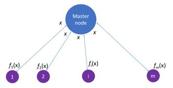
Solving  $\min_{x \in \mathbb{R}^n} \frac{1}{m} \sum_{i=1}^m f_i(x)$  in a master-slave architecture with a master node and m workers. The master node is responsible for maintaining the decision vector x, Each worker i is responsible for processing the function  $f_i$  given the state x (typically computes the gradient  $\nabla f(x)$ ).
