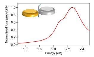
Figure 2: Modelled EEL spectrum of a heterodimer composed of a gold nanodisc (diameter d = 105 nm and thickness t = 25 nm) and a silver nanodisc (diameter d = 105 nm and thickness t = 30 nm). The EEL spectrum is computed for an electron passing through the nanogap center using the standard formalism.
