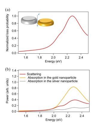
Figure 3: EELS of a heterodimer composed of a gold nanodisc (diameter d = 105 nm and thickness t = 25 nm) and a silver nanodisc (diameter d = 105 nm and thickness t = 30 nm). (a) The EEL spectrum is computed for an electron passing through the nanogap center using the antenna perspective. (b) The absorbed power in the gold nanodisc and in the silver nanodisc and the scattered power shown as functions of energy loss.
