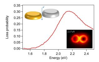
Figure 1: EELS of a heterodimer composed of a gold nanodisc (diameter d = 105 nm and thickness t = 25 nm) and a silver nanodisc (diameter d = 105 nm and thickness t = 30 nm) separated by a 9 nm gap. The EEL spectrum is measured for an electron beam passing through the nanogap center. The inset shows the EELS map for an energy loss of 2.17 eV integrated over a 0.1 eV window.
