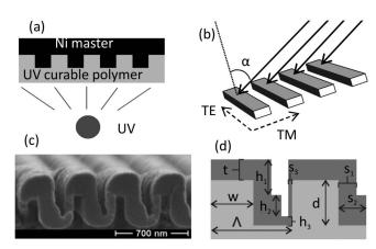
Fig. 1. (a) and (b) Fabrication procedure and orientation of the E-vector with respect to the grating for the two polarizations, (c) SEM picture of the obtained structure, and (d) model used for simulations.
