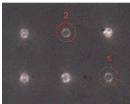
Fig. 5. ( Media 3 ) Optical plasmonic trapping of yeast cells in a microfluidic channel (objective 50 \times ). The bright structures represent the gold disks with trapped yeast cells on top of them. During the movie, a free yeast cell becomes trapped in the bottom right highlighted structure and another cell is trapped by the top highlighted disk about half a minute later.
