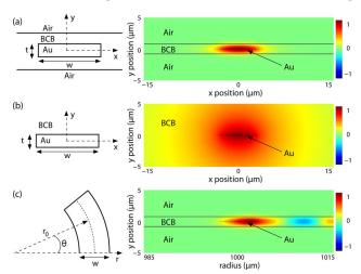
Fig. 1. (Color online) Geometry and  $E_y$  field component for the fundamental long-range mode of (a) a straight Au strip of rectangular cross section ( $w=6~\mu\mathrm{m},~t=10~\mathrm{nm}$ ) in a BCB layer of thickness 1.6  $\mu\mathrm{m}$ ; (b) the same Au strip in an infinite volume of BCB; (c) a curved Au strip of rectangular cross section ( $w=6~\mu\mathrm{m},~t=10~\mathrm{nm},~r_0=1~\mathrm{mm}$ ) in a BCB layer of thickness 1.6  $\mu\mathrm{m}$ .
