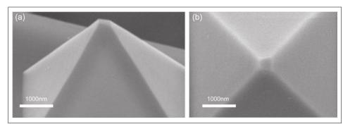
Fig. 6. Towards the next generation of probes. (a): Side view and (b) top view of  $\mathrm{Si}_3\mathrm{N}_4$  AFM tips (scanning electron microscopy images) that have been flattened by laser machining. The flat end face will allow the preparation of much better defined antenna structures in the future.
