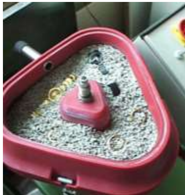
Vibration wear with ceramic chips
