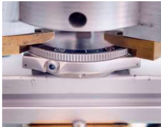
Applying cycles on rotating bezel
