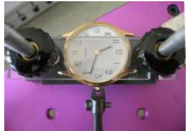
Ageing setting stem (winding, pull-push, date, hand-setting)
