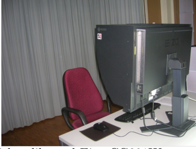
Figure 1: MMSPG test room with calibrated Eizo CG301W screen and controlled lighting system.
