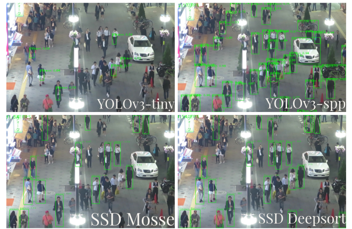
Fig. 3. Comparison of the algorithms. SSD MOSSE : the fastest; YOLOv3-spp : the most accurate; SSD Deep SORT : the only one to "track" people.
