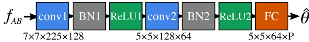
Fig. 3. Feature regression module used by Rocco et al. The output dimension P may be equal to 6 for AFF transformation, or 18 for TPS transformation.
