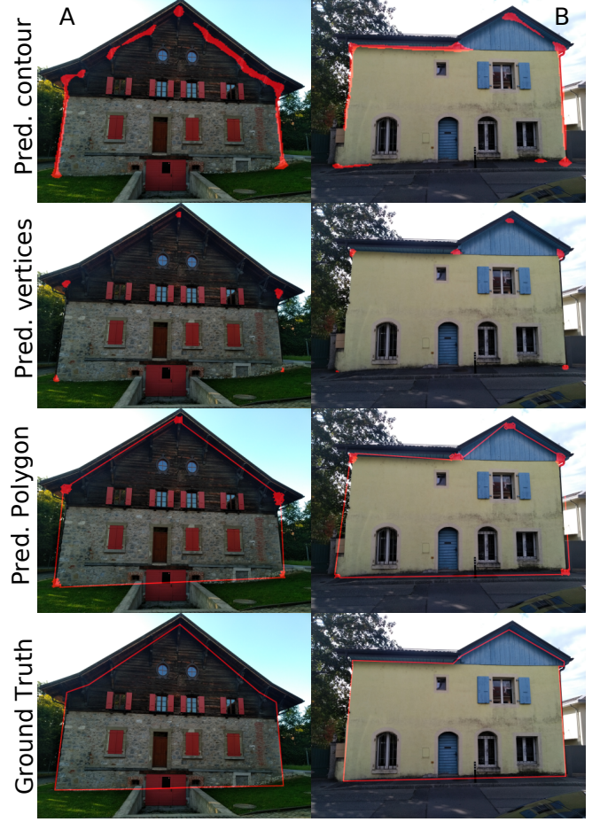
Figure 4. Predictions for U-Net11 model 3, semantic segmentation of the facade contours and vertices, and generating polygons from the vertices.
