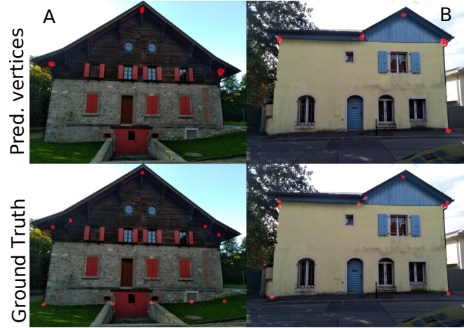
Figure 3. Predictions model 2. Semantic segmentation of facade vertices.
