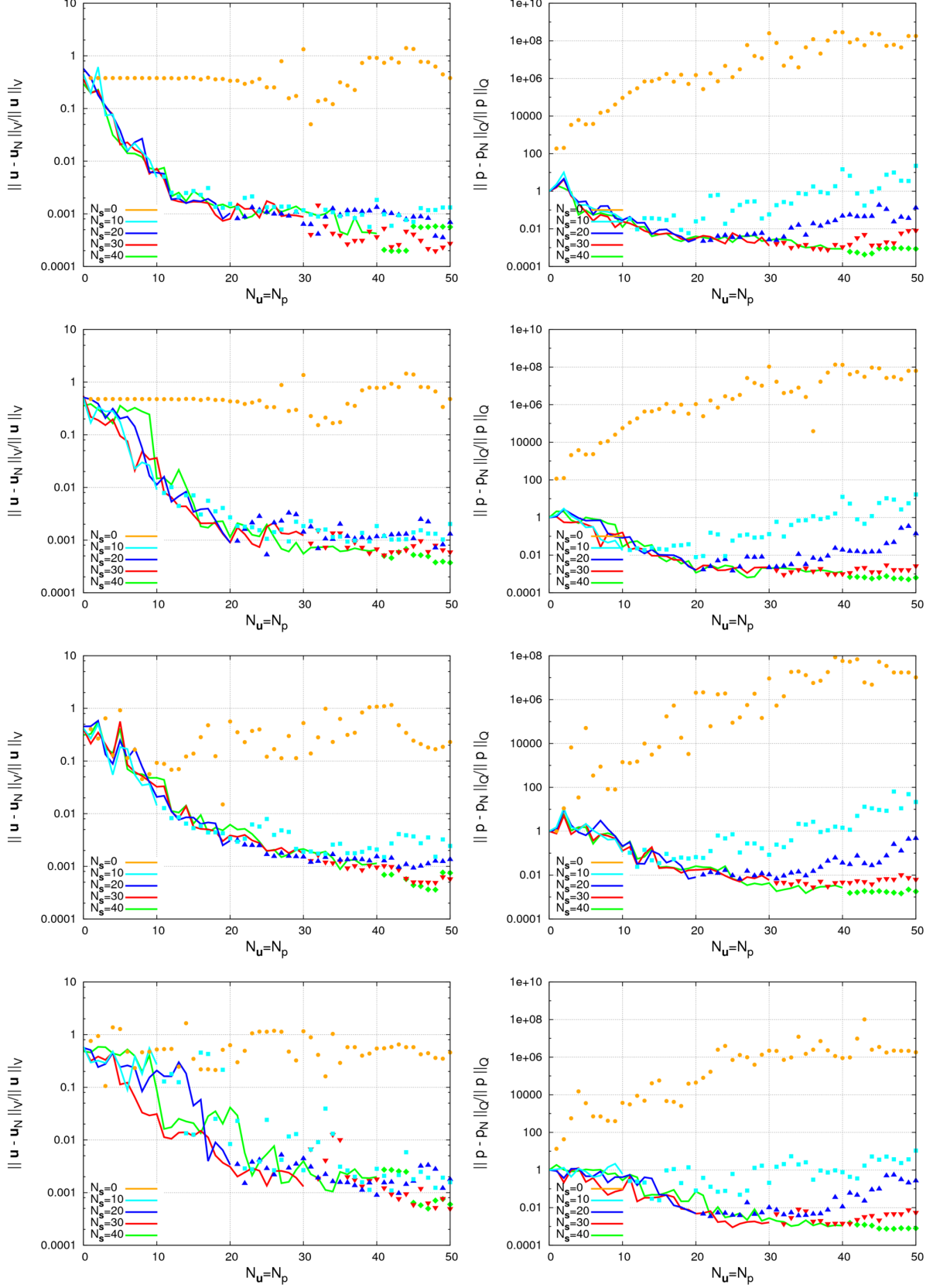
FIGURE 9. Case II – physical and geometrical parameters: error analysis on velocity (left) and pressure (right) components. From top to bottom: ( Re = 90 , H_o/H = 1 ), ( Re = 150 , H_o/H = 1 ), ( Re = 150 , H_o/H = 0.5 ), ( Re = 150 , H_o/H = 1.5 ).
