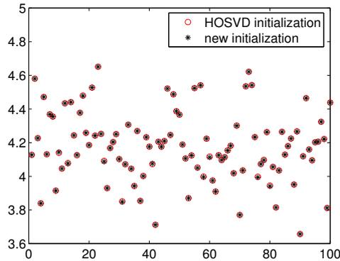
Figure 4: Approximation error of multilinear rank-4 approximation produced by HOPM for 100 random antisymmetric  $10 \times 10 \times 10 \times 10$  tensors.
