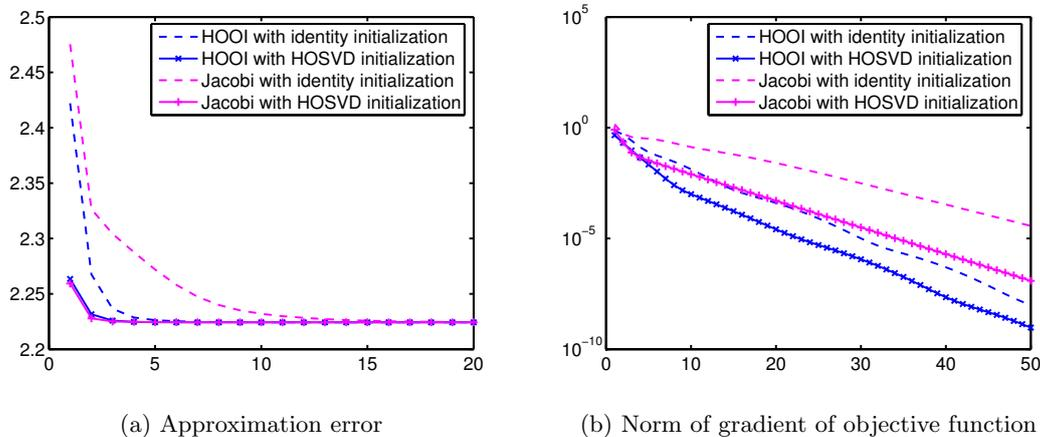
Figure 2: Convergence behavior of HOOI and Jacobi algorithm for multilinear rank-6 approximation of random antisymmetric  $10 \times 10 \times 10$  tensor.
