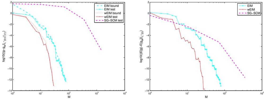
Figure 4.2: Comparison of convergence property of EIM, wEIM and SG-SCM in different norms. Left: decreasing of the error  $\|g - g_M\|_{L^\infty(D; C^0(\Gamma))}$ ; Right: decreasing of the error  $\|\mathbb{E}[g] - \mathbb{E}[g_M]\|_{L^\infty(D)}$ .
