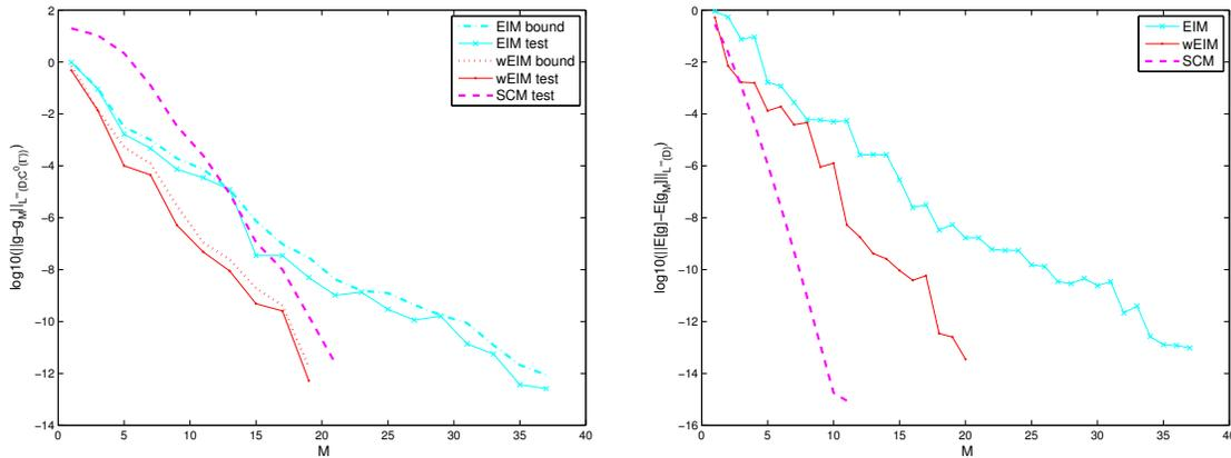
Figure 4.1: Comparison of convergence property of EIM, wEIM and SCM in different norms. Left: decreasing of the error  $\|g - g_M\|_{L^\infty(D; C^0(\Gamma))}$ ; Right decreasing of the error  $\|\mathbb{E}[g] - \mathbb{E}[g_M]\|_{L^\infty(D)}$ .
