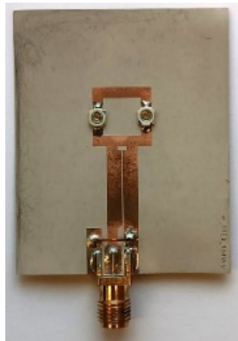
Fig.1. Example of antenna.
