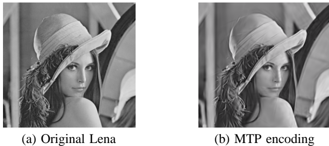
Fig. 8. The Lena image (256x256) encoded with the MTP sample algorithm at 0.41bpp [PSNR = 32.73dB].
