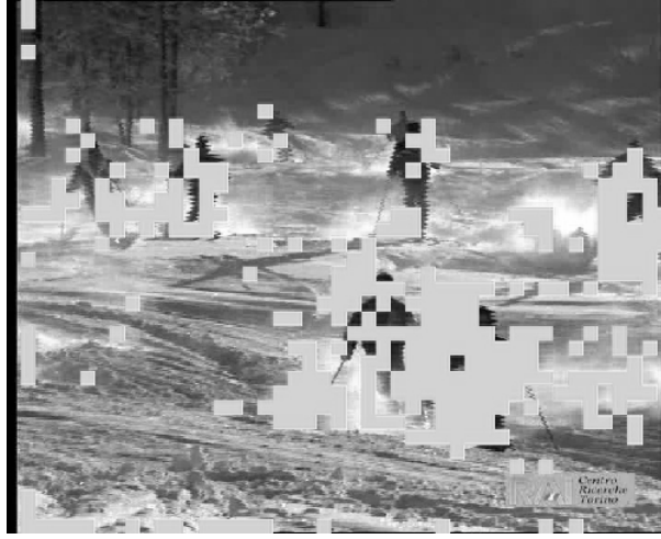
FIGURE 5.7: Sample frame of ITU-R test sequence, where AMISP additional Intra-macroblocks are designed in light gray.
