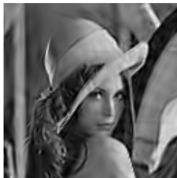
FIGURE 9.4: Matching Pursuit coded Lena image of size 256 \times 256 with 500 iterations decoded at a resolution of 128 by 128 pixels (PSNR = 25.42 dB).
