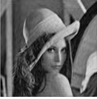
FIGURE 8.11: Reconstruction of the Lena image with Gabor atoms after 1000 MP iterations (PSNR = 31.17 dB).
