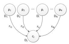
**Fig. 4.** Peer node  $c_j$  desires a set of descriptions  $D_j$ , while its parents  $p_i$  are interested in possibly other descriptions  $D_i$ . The link capacity for a link connecting parent  $p_i$  with  $c_j$  is equal to  $r_{ij}$ .
