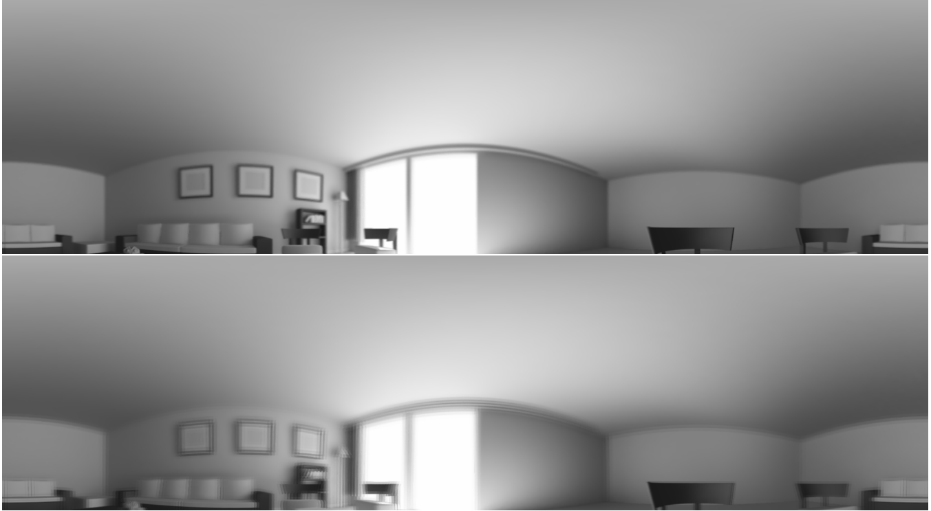
Fig. 3. Reconstruction results with focus plane on the closest object, the chair on the bottom right of the image. Top: the sampling conditions are respected. Bottom: the sampling conditions are not respected and artifacts in the form of double lines are visible in the image.
