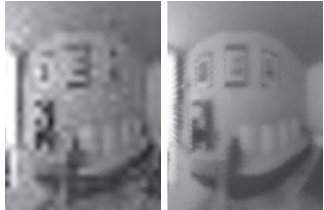
Fig. 4. Zoom on a detail: on the left the LR image (64x64) we use in the reconstruction. On the right the reconstructed HR image (512x512) using 12 images with estimated registration.
