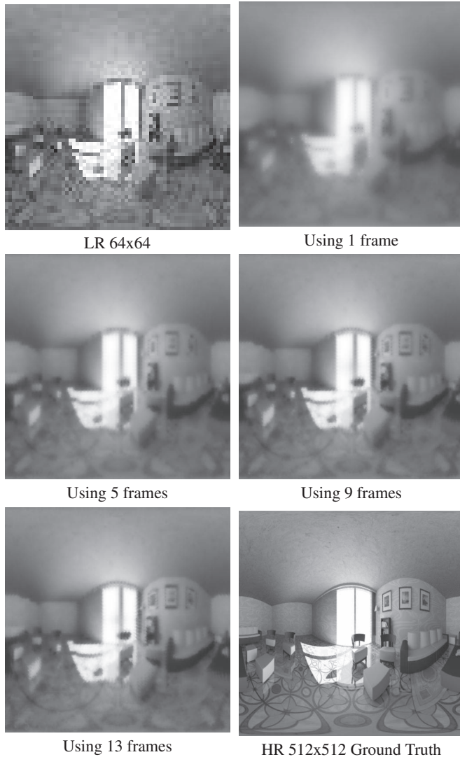
Fig. 3. Visual results using increasing number of frames (1,5,9,13) from the 64x64 video sequence. Top left: the LR image. Bottom right: the HR ground truth image.
