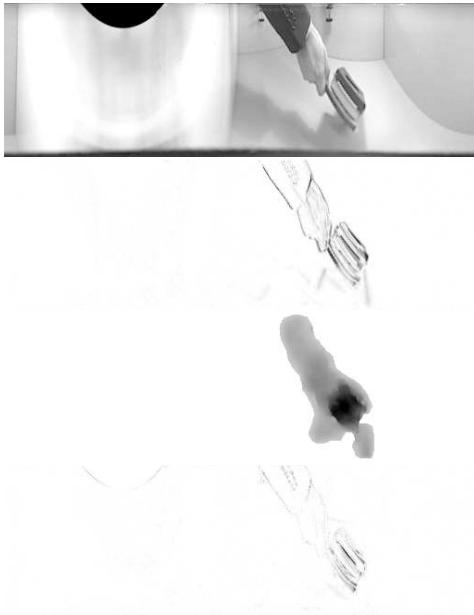
Fig. 4. Optical flow estimation from catadioptric images. From Top to bottom: image after projection on the sphere; frame difference I_1 - I_0 ; optical flow field (module); image residual I_1(\mathbf{x} + \mathbf{u}) - I_0 , after motion compensation.
