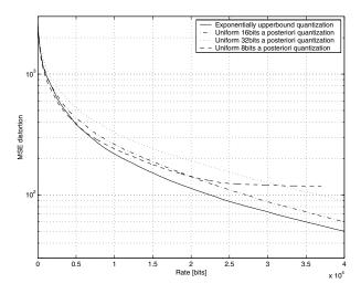
Fig. 2. Rate-distortion curves for the new quantization scheme and uniform a posteriori quantization of Lena MP stream. Distortion is represented as a function of the total rate.
