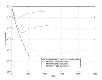
Fig. 1. R-D curve for the decomposition of a random signal of length 10 over a random dictionary of 50 vectors. Comparison of exponential quantization and uniform quantization as a function of the total rate.
