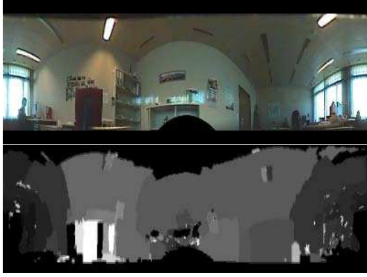
Fig. 10. Reference image and disparity images a graph-cut method on the sphere [35].
