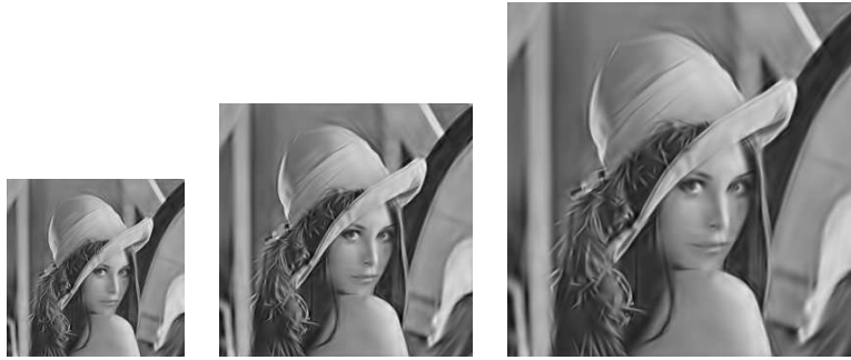
Figure 3. Lena image of size 256 \times 256 encoded with MP at 0.3bpp (center), and decoded with scaling factors of \sqrt{\frac{1}{2}} (left) and \sqrt{2} (right).
