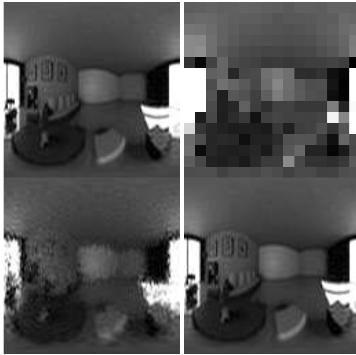
Fig. 3: Groundtruth high-resolution image (top-left), one low-resolution image (top-right), reconstructed image with registration errors, PSNR = 24.30 dB (bottom-left), reconstructed image with the Levenberg-Marquardt algorithm. PSNR = 44.28 dB. (bottom-right).
