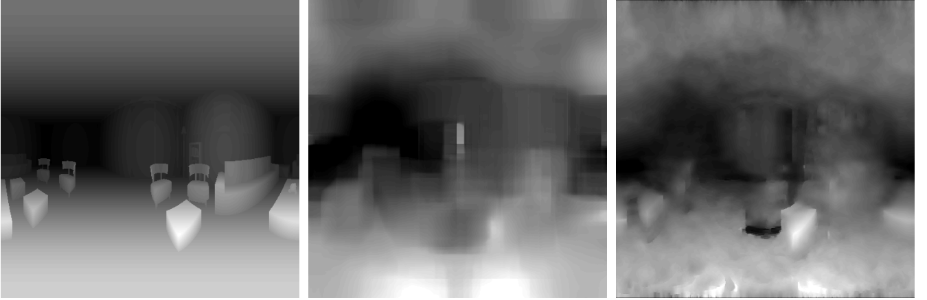
Fig. 10. Depth estimation performance for LK (middle) and TV-L1-GrH (right) algorithm, compared to the ground truth depth map (Left).
