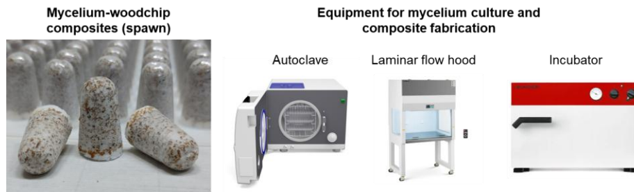
Figure 2. Image of the mycelium-woodchip composites (left) and the equipment required for the composite fabrication (right).
