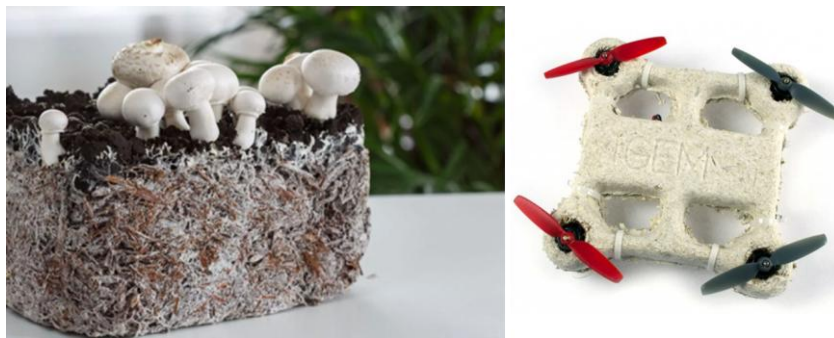
Figure 1. Image of mushroom (mycelium and fruiting bodies) (left) [1] and previously reported biological UAV made of fungus-like materials (right) [2] .
